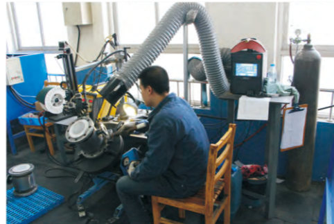
Flowmeter Welding Process
